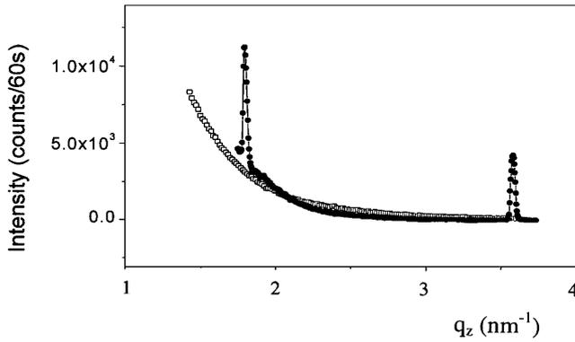
**Fig. 1.** X-ray intensity profiles as a function of  $q_z$  for a  $10\ \mu\text{m}$  thick film with  $P_w = 55$  in the  $\text{Sm-A}_d$  phase. Open squares: annealed at  $T = 115\ ^\circ\text{C}$ ; filled dots: annealed at  $T = 93\ ^\circ\text{C}$ .
