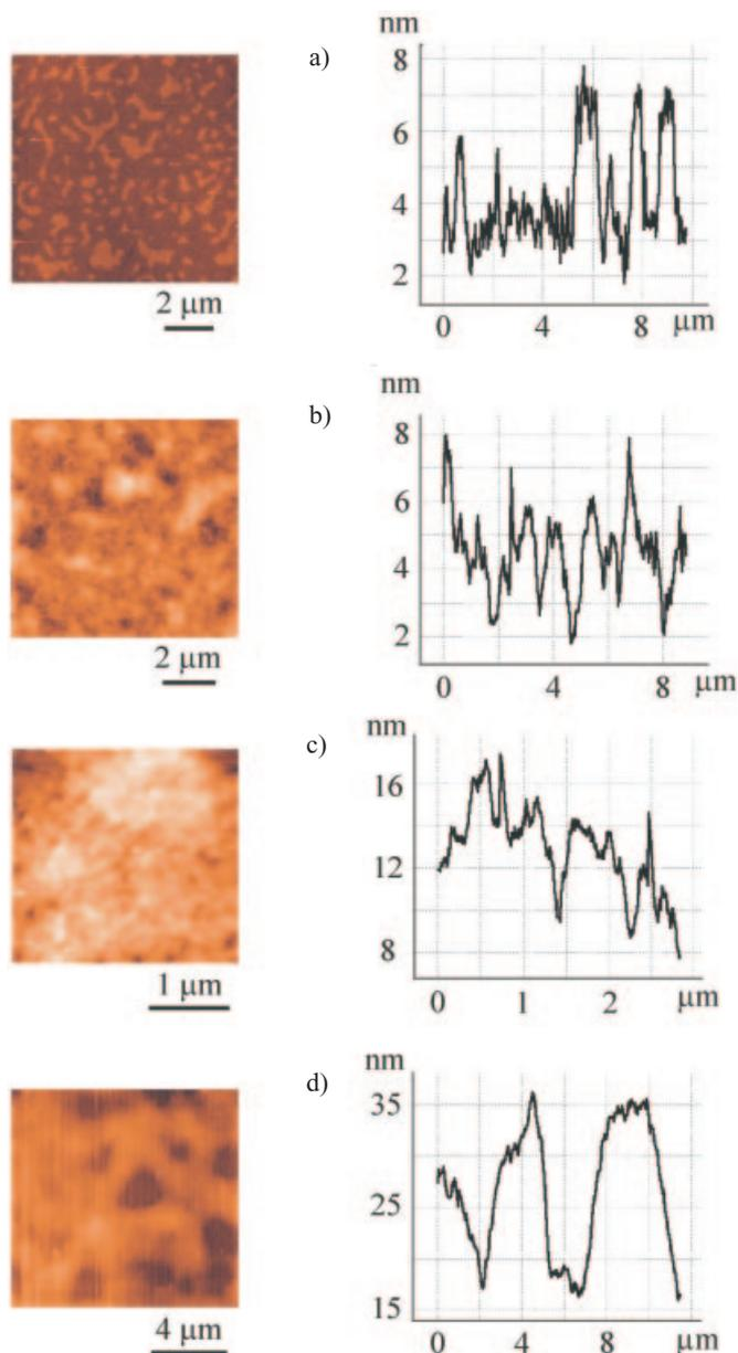
**Fig. 3.** AFM images for a 28 nm film with  $P_w = 55$ . (a) Annealed at  $T = 105^\circ\text{C}$  in the Sm-A $_d$  phase ( $1.5 \times 1.5$   $\mu\text{m}^2$ ). The contrast corresponds to terraces with an average thickness of  $\sim 3.5$  nm. (b) Annealed at  $T = 75^\circ\text{C}$  in the RN phase. (c, d) Annealed at  $T = 53^\circ\text{C}$  in the  $\tilde{C}$  phase (different stages of dewetting are shown).
