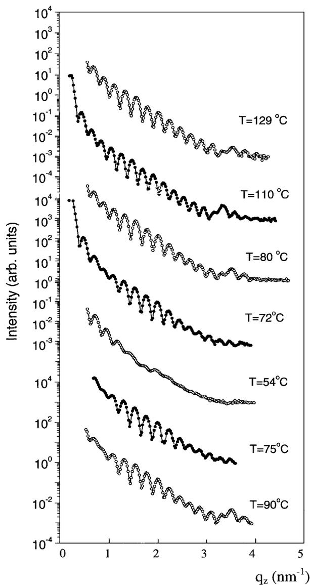
**Fig. 2.** X-ray reflectivity of a 28 nm film with  $P_w = 55$  as a function of  $q_z$  at the temperatures indicated. Curves have been shifted for clarity.
