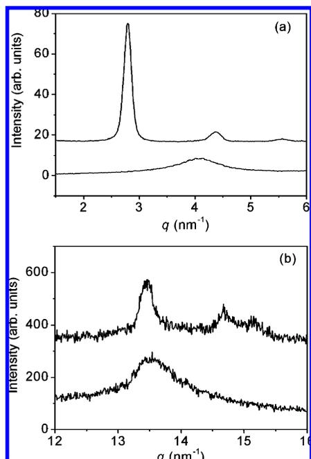
**Figure 2.** SAXS (a) and WAXS (b) patterns for  $C_8Ch$  for the Col<sub>rp</sub> (top) and N (bottom) phases. Curves have been shifted for clarity.
