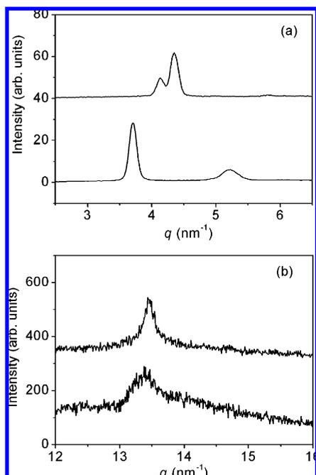
**Figure 5.** SAXS (a) and WAXS (b) patterns for mh-Ch at 290 °C (upper) and eh-Ch at 170 °C (lower). Curves have been shifted for clarity.
