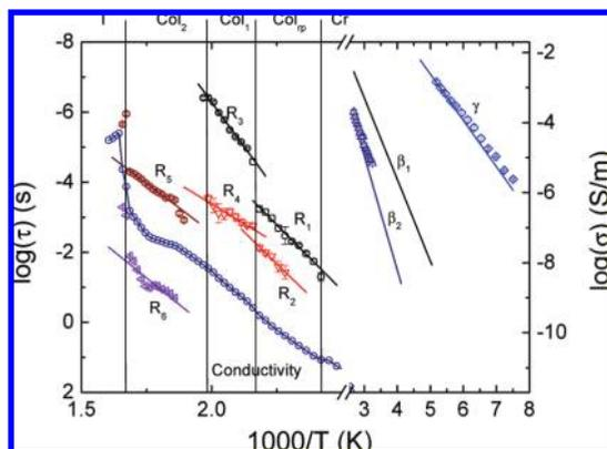
**Figure 8.** Activation plot for all dielectric relaxation processes in eh-Ch (relaxation time  $\tau$ , left axis) and conductivity ( $\sigma$ , right axis) as a function of inverse temperature.<sup>38</sup> The relaxation processes are labeled as in Table 5, and the phase regions are indicated by vertical lines and labeled on top.
